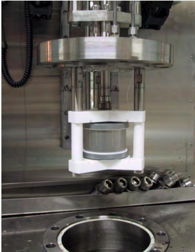
cage (RC) are used to study corrosion inhibitors in oil and refinery environment as described in **ASTM G170**.
