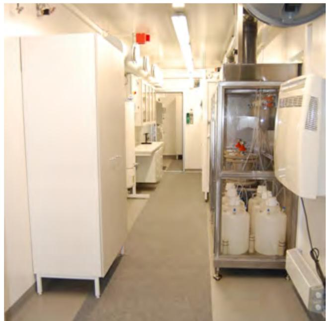
A R&D or H2S quality assurance laboratory can be built in a house or in a container. A container is a potential alternative to a conventional house lab, because as a separated unit it can be better isolated from the environment in terms of ventilation and poisonous gases such as H2S and CO2. If needed, a container lab can also be moved easily, for example if testing requires connection to a plant's process flows or presence close to pipe factory. A container laboratory will be fully instrumented
